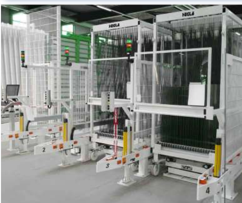
Slot Carriage Station for continual glass provision for the subsequent processes
