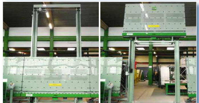
Vertical conveyor with lifting unit: Quick-opening passage and through-transport.
