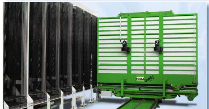
Output-Shuttle: Automatic acceptance of one or more panes from the dynamic storage system.
