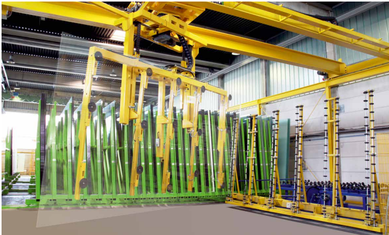
PBD 6133 Gantry Loading System with rotatable vacuum frame for flexible loading, either in front or comp-through, from any storage location. The System is available as Gantry, Semi-Gantry or in overhead-crane design
