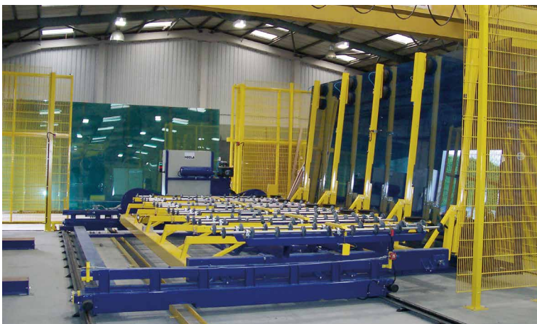
BBF 6133 Sheets are taken from storage-racks by the static or moveable HEGLA Floor-loader type EBS/BBS or EBF/BBF. The moving type system can facilitate up to 6x2 positions (racks).
