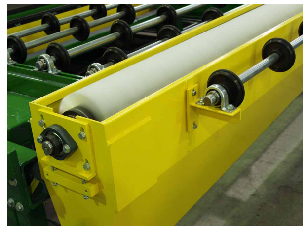
Brush roller with catching-container for cleaning-off the Lucite from the lower glass surface. Vacuum extraction unit available optionally.
