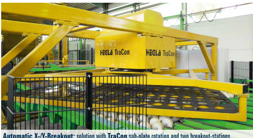
Automatic X-Y-Breakout: solution with TraCon sub-plate rotation and two breakout-stations
