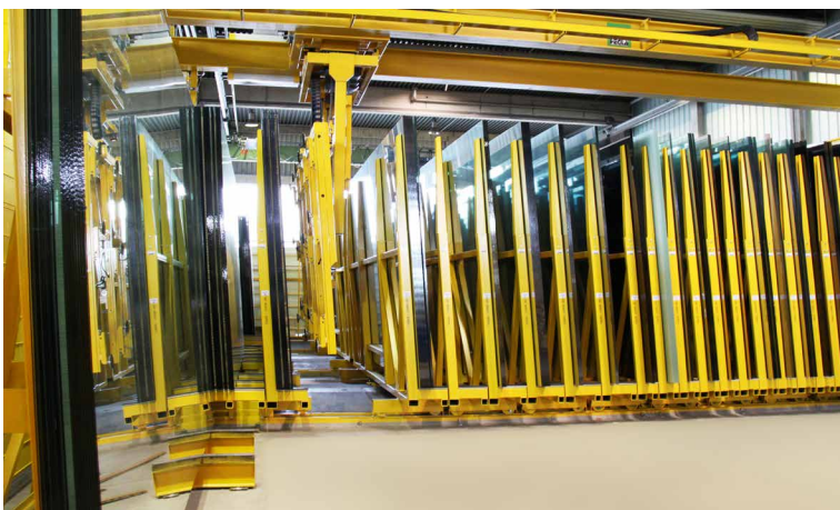
KPL-A The automatic compact storage system utilizes the available space to its maximum and enables automatic loading and storage with a Gantry Loader or the Compact Loader.
