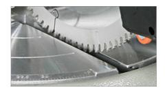
Cutting unit with carbidetipped or high speed steel blade
